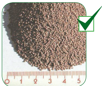
5g approx. 35,000 microgranules – average diameter of 0.7 mm (low dust level!).
