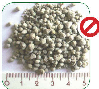
5g of general NPK: approx. 330 granules – average diameter of 3.3 mm .
